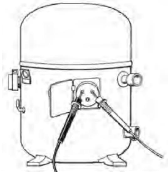
When measuring resistance of a motor, make sure the power is disconnected prior to testing.
