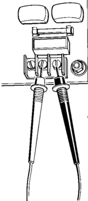
Disconnect power from the terminal block, find the fuse or circuit breaker that controls the block and turn it off.
