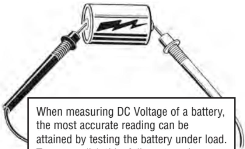
When measuring DC Voltage of a battery, the most accurate reading can be attained by testing the battery under load. To accomplish this, follow steps 1 through 4 shown on page 14 and the following (with the battery in holder and device turned on):
